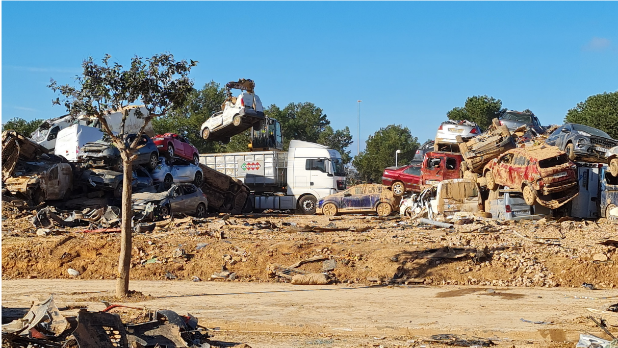
Fig. 3 Loading of cars with gripper arm, without pumping out hazardous substances and removing batteries (Stephan Müllers)
